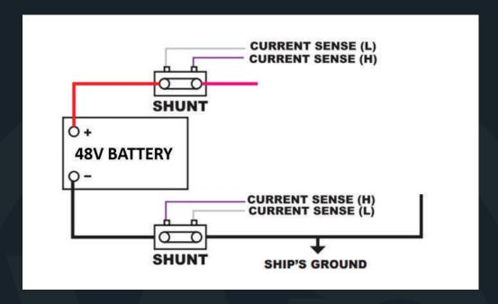
**Note:** Diagram is intended to indicate placement of current sense wires base on shunt location. Only one shunt is required for regulator operation.
